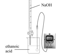
A sodium hydroxide solution was titrated with a solution of ethanoic acid using the apparatus shown on the right. A number of pH readings, together with the corresponding volumes of sodium hydroxide solution added, are shown in the table.
