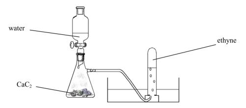
water dropping on to / tap (dropping) funnel containing water //
